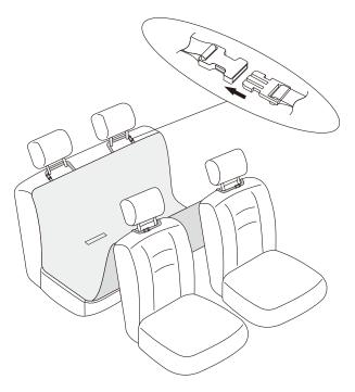
Set the straps around the headrest, adjust the 4 plastic clips to fix cover firmly.
