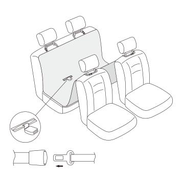
Open the Velcro, pull out the seat belt buckles. Put one end of the safe belt in the buckle clasp.
